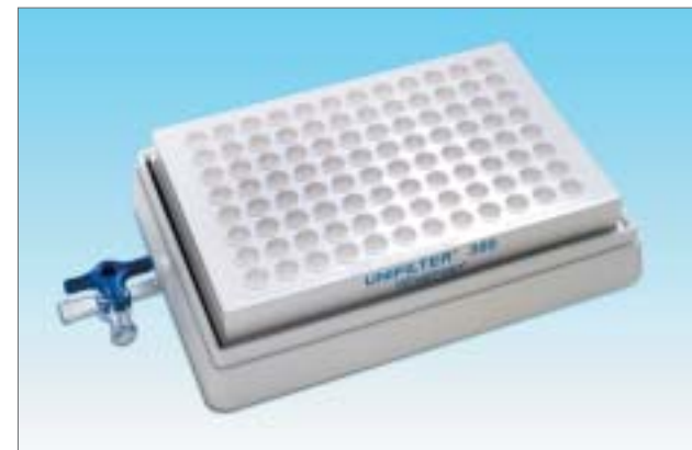
UniVac 1 Vacuum to Waste Manifold
